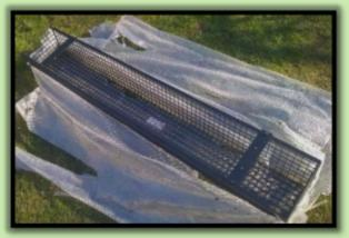
1 x Anti Roll Bar Kit Assembly for a Snatch 2 made by Ricardo. It looks like everything is there to complete the job... The anti roll bar, two mounting rubbers, the two plates that weld to the axle and a set of bolts. £120
